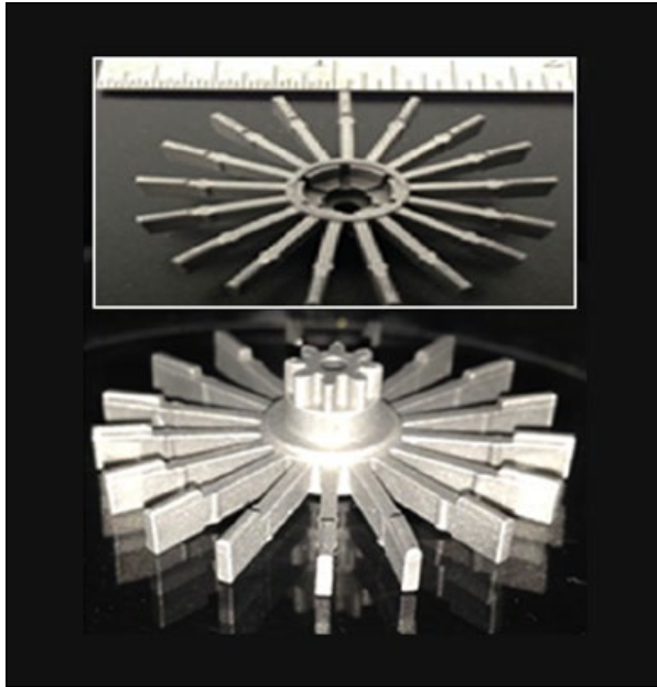
Fig. 2 Aluminium MIM sample part manufactured by Ryer Inc. using the aluminium 6061 feedstock
